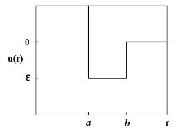
FIG. 1. Square-well potential. The ratio of the attractive distance b to the hard-core repulsive distance a is  $b/a = \sqrt{3}$ . The depth of the square-well  $\epsilon = -1.0$  is the interaction energy per pair of particles.
